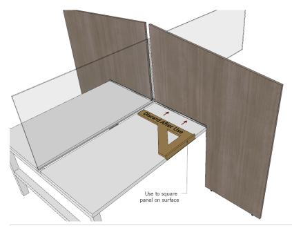
Locate Panel Divider in place and use provided square template to position panel and lower floor glides to level the panel.
